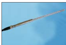
RFTXS-325 - miniaturised sensor for measuring for example in screed. max. +80°C D=4,6mm, L=200mm,
