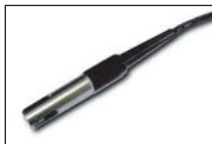
RFT-325 - Measures humidity and temperature. Operating range: -20 and +80°C, or -40 to +120°C with cable type G. Dimensions: d=8x35mm
