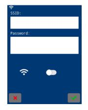
Write the WIFI network in the SSID text box and the password in the Password text box.
