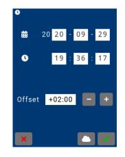
The SC202 allows to set the date and time manually or automatically.
