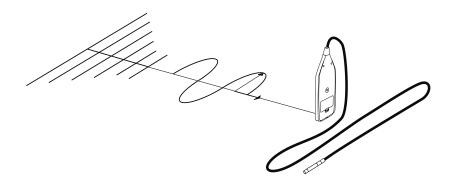
The sound level meter complies with the basic specifications of IEC 61672-1 on the immunity required for fields at the frequency of the alternating power supply (50Hz and 60 Hz) and radio frequency fields
