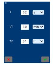
Write the desired time in each text box and then click on the drop-down menu to select the time units (seconds, minutes or hours).
