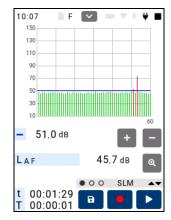
The 1/1 Analyser Screens show in real time the equivalent continuous sound pressure level in octave bands centred on frequencies 8, 16, 31.5, 63, 125, 250, 500, 1000, 2000, 4000, 8000 and 16000 Hz (without frequency weighting). Simultaneously, they show the equivalent global level with the frequency weightings (A, C and Z). They also show the background noise of rooms: NC (Noise Criterion) and NR (Noise Rating) curves.
