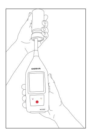
Turn on the calibrator and check the battery status. The LED indicator must remain lit throughout the entire calibration process (see the calibrator manual). The calibrator generates a 94 dB tone at 1 kHz.
