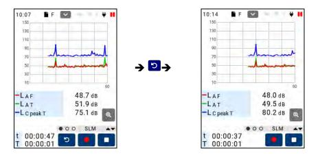
The BACKERASE option is available on any display screen while measuring or recording is temporarily stopped **II** / **II**.
