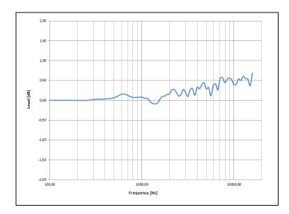
Correction for the average effects of the *PV009* windscreen on the frequency response of the sound level meter in the absence of wind:
