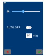
To set the brightness of the screen, move the slider until the desired brightness is achieved.
