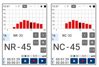
The Analyser Screen (1/3) displays in real time, for the entire dynamic measurement range, the equivalent continuous sound pressure level in the 1/3 octave bands from 6.3 Hz to 20 kHz (without frequency weighting). Simultaneously, it shows the global equivalent level with frequency weighting A, C and Z.
