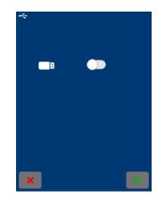
For the SC202 behaves as a mass storage device when it is connected to the PC, the USB option must be enabled.
