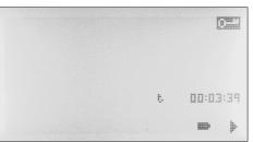
While the keypad is blocked, the values of the functions measured do not appear on the screen, to avoid the deliberate generation of noise to distort the measurement.
