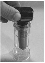
Figure 2-5: Insert Alcohol Cartridge into Fill Capsule
