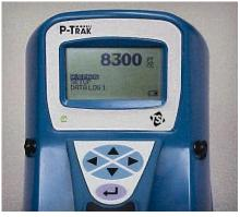
Figure 3-1: P-Trak Particle Counter Keypad and Display
