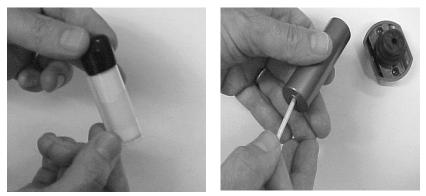
Figure 4-2: Remove Wick and Screen Using Dowel
