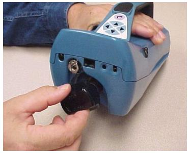
Figure 2-6: Insert Alcohol Cartridge into P-Trak Particle Counter
