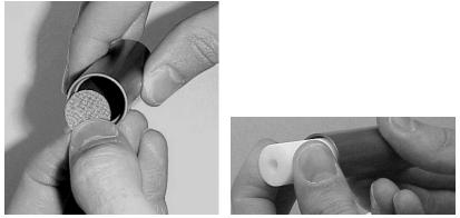
Figure 4-3: Install Screen and Wick into Retainer
