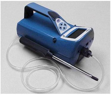
Figure 2-8: Slide Telescoping Probe onto Instrument Case
