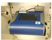
Attach the Dustrak monitor to the tray with the Velcro<sup>®</sup> strap.
