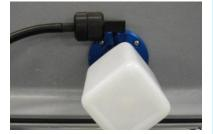
3. Install the Heated Inlet on top of the Auto-Zero Module.
