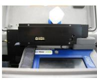
Attach inlet tube to Heated Inlet.
