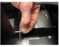
6. Attach the Mounting Bracket to the Heated Inlet with 8-32 thumbscrews—do *not* tighten.
