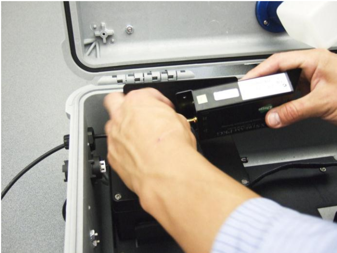
Figure 12: Attach Antenna and Cable to Radio Modem
