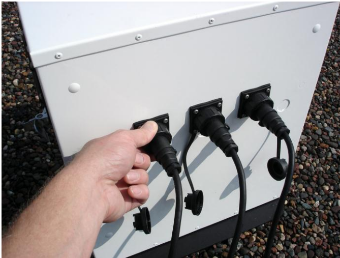
Figure 49: Connect Power from the Solar Cell Power System to the Environmental Enclosure
