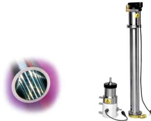
DMA's contain highly polished surfaces for high-resolution particle size classification (left). The Series 3080 offers a choice of two DMA's (right).
